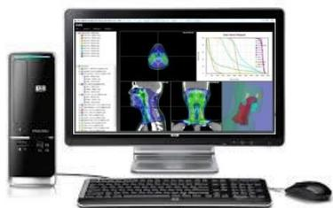
This viewer can show dose mapping and structures from all radiotherapy planning system. 3D graphic and dose-volume histogram (DVH) is achieved by high-speed processing system.
